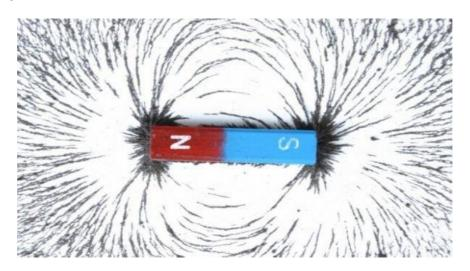
This is a magnet. Magnetic lines are made livable by spreading iron filings around the body producing a magnetic field.
